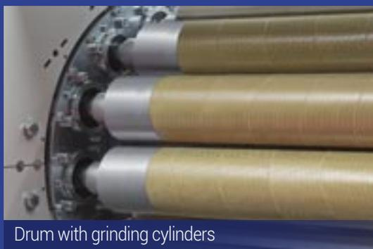
Drum with grinding cylinders
