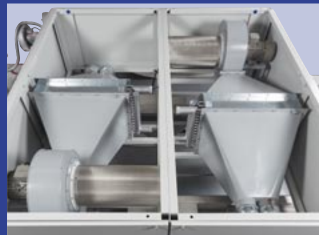
Thermal exchangers for selvedges drying
