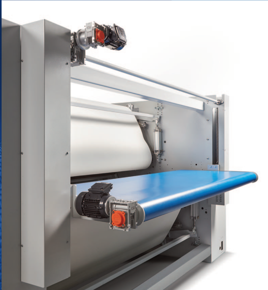
Movable by-pass device between the first and second compaction module
